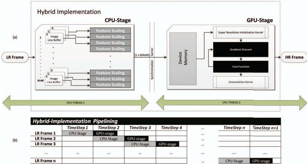
Fig. 1. (a) The Hybrid Implementation Flowchart (b) The Hybrid Implementation Pipelining. By splitting the overall algorithm and assigning different parts to two separate resources enables us to pipeline the procedure. The experimental results have confirmed that for systems armed with powerful CPUs compared to their GPUs abilities, the pipeline approach succeeds a reduction of the overall execution time compared to the GPU-only implementation, more evident in small image sizes.
